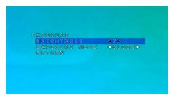
In this menu item you can first adjust the overall brightness of the picture BRIGHTNESS. Then you can choose the exposure mode EXPOSURE MODE.
