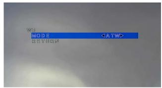
The white balance options are MODE ATW (the white balance is automatically adjusted to vary the type of lighting) and MODE MWB (manual setting of the white balance by changing the values in RGAIN and BGAIN entries)
