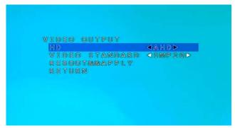
The menu items to be targeted are HD, to choose the technology (AHD, TVI, CVI, CVBS); VIDEO STANDARD, to choose the resolution (5MP20, 5MP12.5, 4MP25, 4MP30, 4MP15, 1080p25, 1080p30); REBOOT & APPLY to confirm the adjusted settings and reboot the camera with the new settings.
