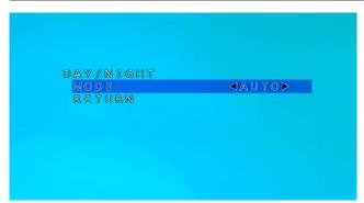
The AUTO setting is always recommended for cameras with built-in IR.
